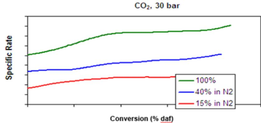
Effect Of Operating Pressure On Reaction Rate
