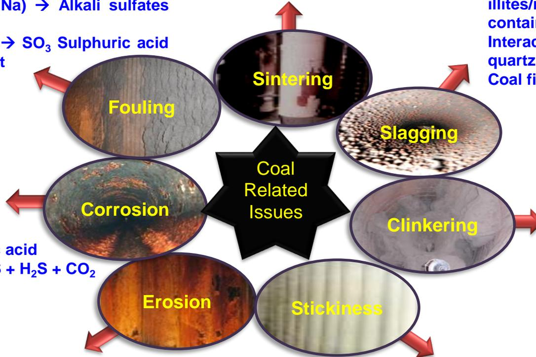
Extraneous rock fragments (Eg. Sandstone, siltstone, mudstone and carbonaceous shale) + Free aluminium silicates (Clays) → Molten agglomerates
