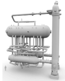
Process Gas Boiler, Heat Recovery System
